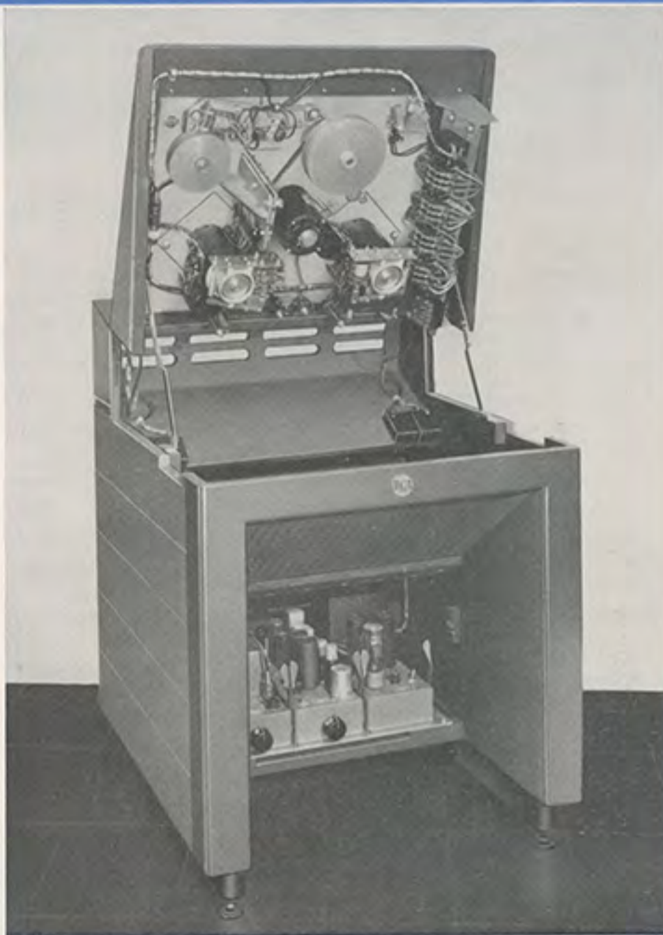
Above, view of Type RT-12B Professional Tape Recorder with top raised and bottom panel removed, showing full access to all components.
