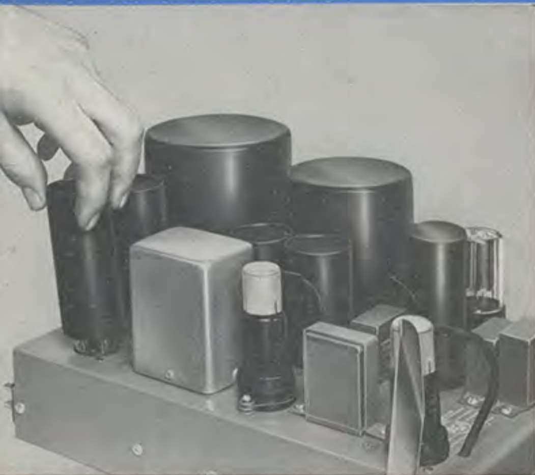
"Plug-in" type electrolytics provide long-life operation and maximum accessibility.
