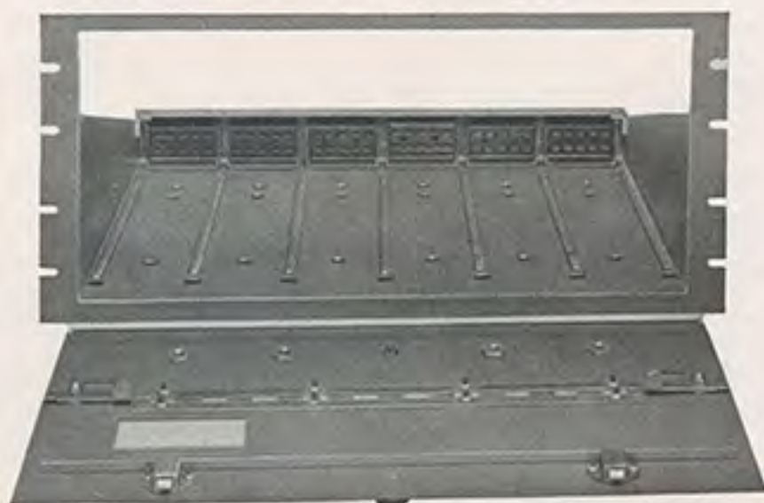
Panel removed showing guide bars and receptacles.
