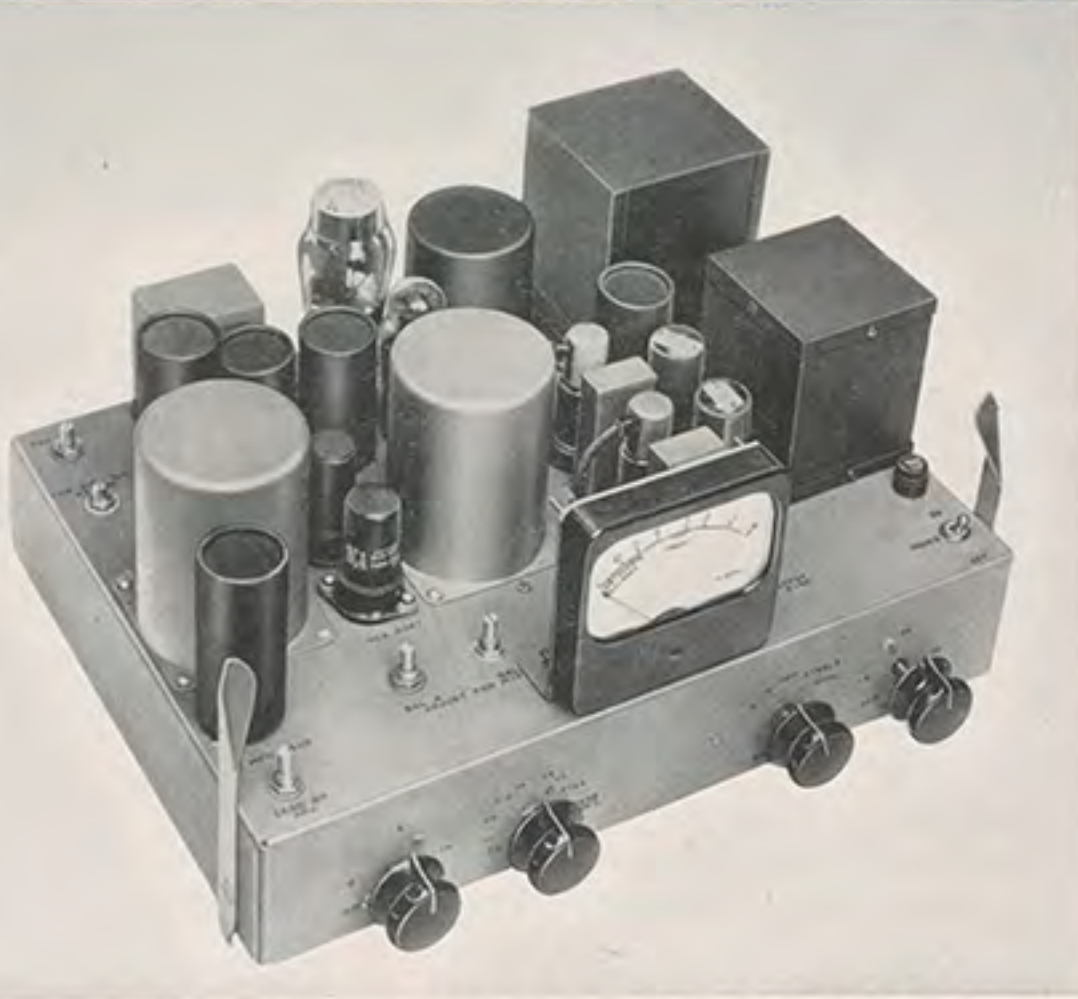
Limiting Amplifier chassis showing position of components
