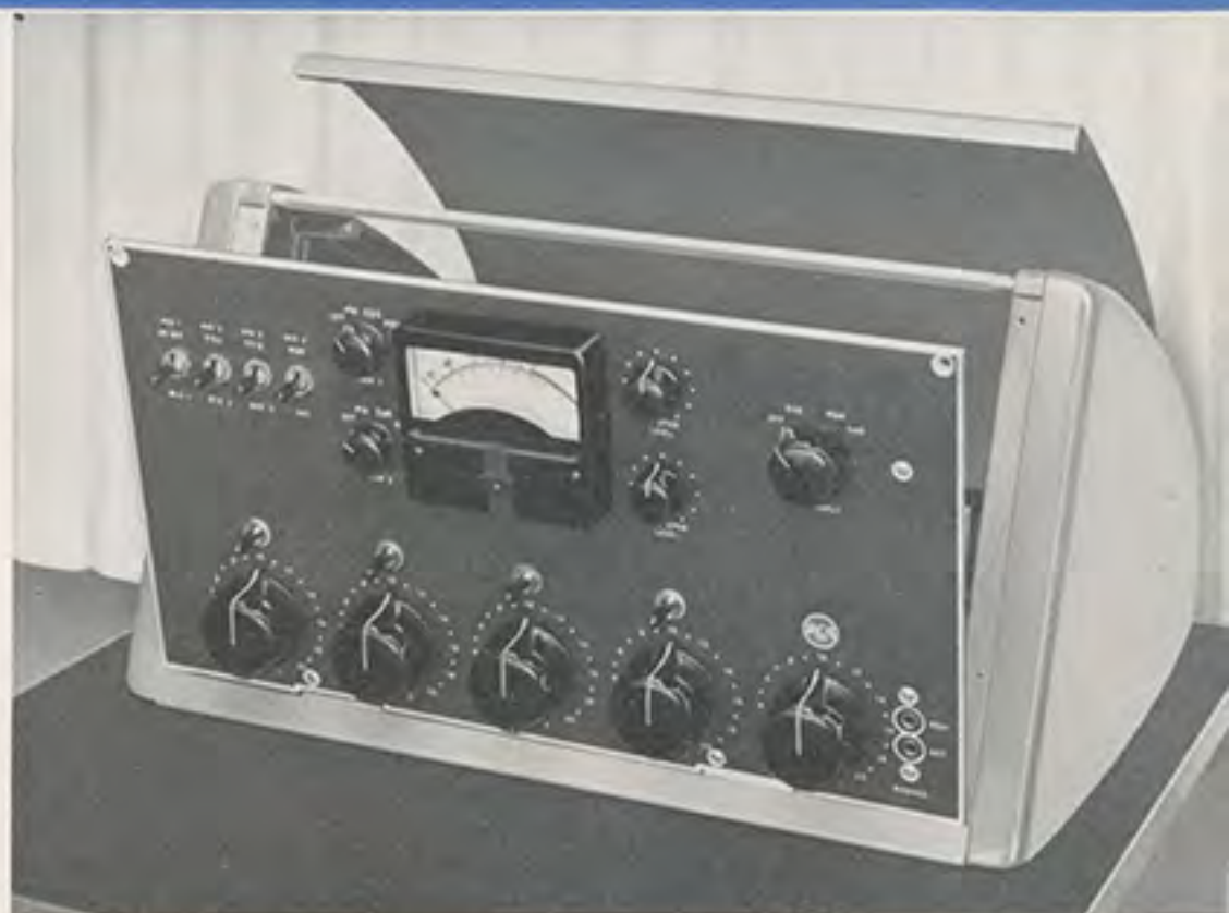
The BC-4A hinged front panel and removable back cover provide complete access to all components and wiring.
